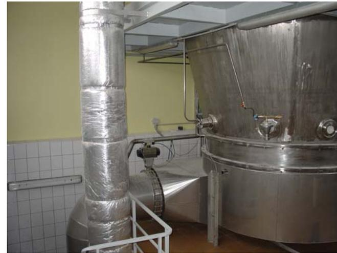
Fluid bed dryer substructure
